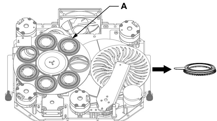
b). Use tweezers or other small grippers to remove the snap spring at point **B** (If the pattern piece is coated with glass glue for fixation, please use a professional cleaning agent to remove the glass glue before removing the snap spring to avoid damaging the gobo);
