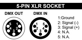
The lighting fixtures are equipped with standard DMX XLR input and output sockets. Please use DMX512 shielded twisted pair signal cables or Category 5 or above network twisted pair cables for connection. The typical connection distance for DMX signal lines is 150 meters. When transmitting signals over long distances, a DMX512 signal amplifier must be added.
