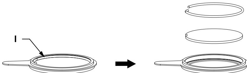
g). When assembling the gobo, avoid touching it directly with your hands. As shown in **J**, align the notch of the gobo with the recess of the driven wheel component (the coating surface of the gobo should face the light source);
