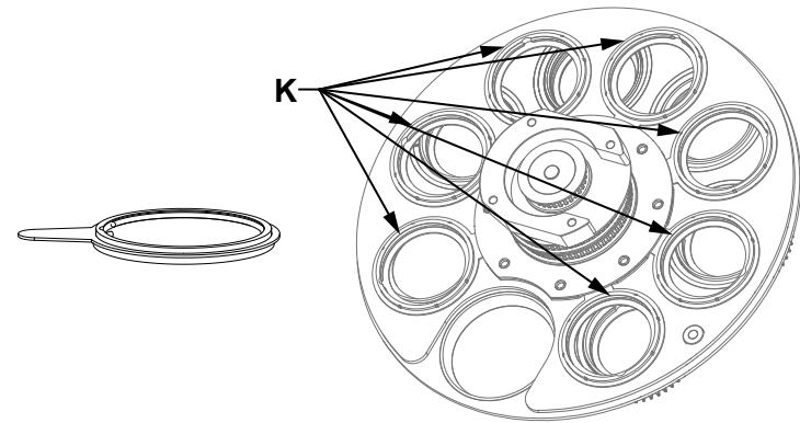
i). After installation, simply reinstall the gobo wheel component onto the light fixture.
