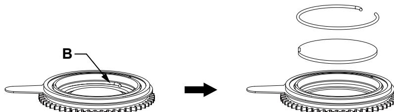
c). When assembling the gobo, avoid touching it directly with your hands. As shown in **C**, align the notch of the gobo with the recess of the driven wheel component (the coating surface of the gobo should face the light source);
