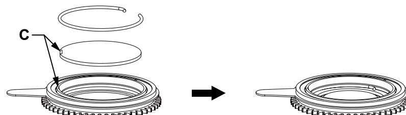
d). Insert the gobo wheel into the drive wheel assembly, as shown in **D**, and reinstall the gobo holder in the order it was removed. After installation, simply reinstall the gobo wheel component onto the light fixture.
