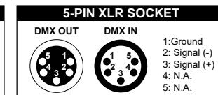
The lighting fixtures are equipped with standard DMX512 input and output sockets. Please use DMX512 shielded twisted pair signal cables or Category 3/5 or above network twisted pair cables for connection. The typical connection distance for DMX signal lines is 150 meters. When transmitting signals over long distances, a DMX512 signal amplifier must be added.
