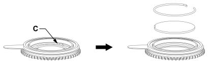
d). When assembling the gobo, avoid touching it directly with your hands. As shown in D, align the notch of the gobo with the recess of the driven wheel component (the coating surface of the gobo should face the light source);
