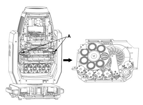
b). As shown in **B**, gently lift the driven wheel from the edge upwards from the front of the pattern plate and slowly pull it out to remove a single pattern seat;
