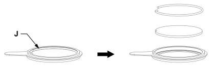
e). When assembling the gobo, avoid touching it directly with your hands. As shown in  $\mathbf{K}$ , align the notch of the gobo with the recess of the driven wheel component (the coating surface of the gobo should face the light source);
