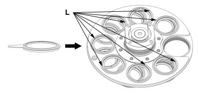
g). After installation, simply reinstall the gobo wheel component onto the light fixture.
