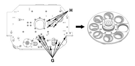
c). As shown in I, gently lift the gobo holder from the edge of the gobo wheel 2 and slowly pull it out to remove a single gobo holder;
