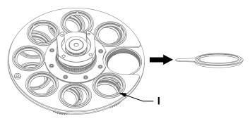
d). Use tweezers or other small grippers to remove the snap spring at point **J** (If the pattern piece is coated with glass glue for fixation, please use a professional cleaning agent to remove the glass glue before removing the snap spring to avoid damaging the gobo);
