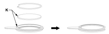
f). Insert the gobo wheel into the drive wheel assembly, as shown in L, and reinstall the gobo holder in the order it was removed;
