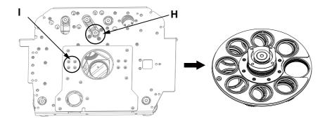
c). As shown in **J**, gently lift the gobo holder from the edge of the gobo wheel 2 and slowly pull it out to remove a single gobo holder;
