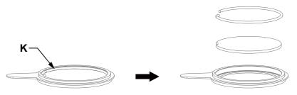
e). When assembling the gobo, avoid touching it directly with your hands. As shown in  $\mathbf{L}$ , align the notch of the gobo with the recess of the driven wheel component (the coating surface of the gobo should face the light source);
