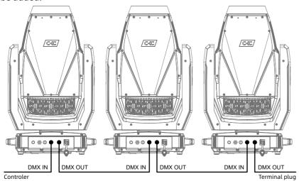
Connect a shielded twisted pair signal cable from the DMX output port of the controller to the DMX input port of the first device, and from the DMX output port of the first device to the DMX input port of the second device, and so on, until all the lamps are connected. Then install a terminal plug on the last 3 pin socket of each connected lamp output. (Weld a 4/1W, 120  $\Omega$  resistor between the 2 and 3 pins of a 3 or 5 core pin XLR plug).
