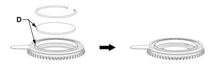
e). Insert the gobo holder into the drive wheel assembly, as shown in **E**, and reinstall the gobo holder in the order it was removed; The positioning point of the gobo holder should be aligned with the positioning point of the driving wheel; After installation, simply reinstall the gobo wheel component onto the light fixture.
