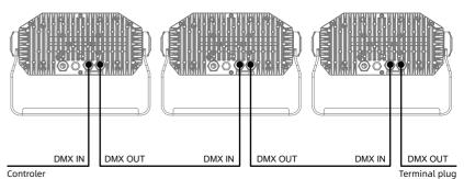
Connect a shielded twisted pair signal cable from the DMX output port of the controller to the DMX input port of the first device, and from the DMX output port of the first device to the DMX input port of the second device, and so on, until all the lamps are connected. Then install a terminal plug on the last 3 pin socket of each connected lamp output. (Weld a 4/1W, 120 Ω resistor between the 2 and 3 pins of a 3 or 5 core pin XLR plug).
