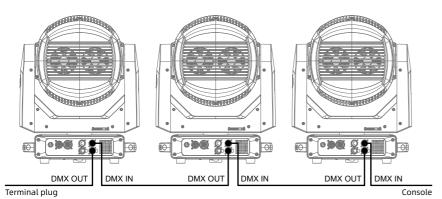
Connect a shielded twisted pair signal cable from the DMX output port of the controller to the DMX input port of the first device, and from the DMX output port of the first device to the DMX input port of the second device, and so on, until all the lamps are connected. Then install a terminal plug on the last 3 or 5 pin socket of each connected lamp output. (Weld a 4/1W, 120 Ω resistor between the 2 and 3 pins of a 3 or 5 core pin XLR plug).
